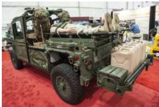
The Corps' Ground Unmanned Support Surrogate (GUSS) can transport gear and casualties for Marines.
