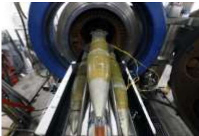
In this Jan. 29, 2015 photo, inert 105mm shells sit in the entry point of the explosive destruction system used for destruction of leaky or otherwise problematic chemical munitions, inside the Pueblo Chemical Depot
