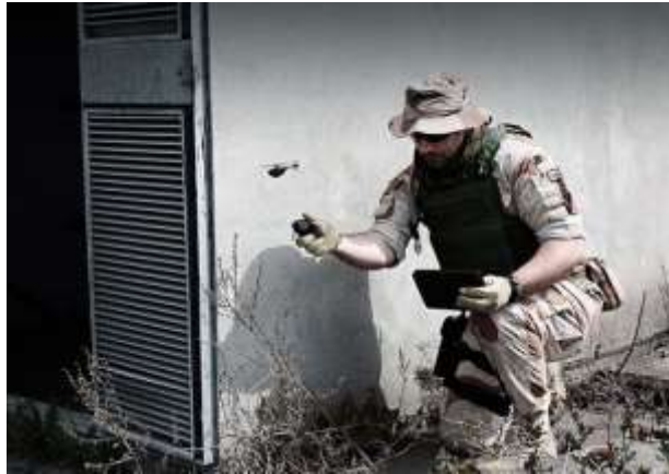
The Marine Corps Warfighting Laboratory is interested in the PD-100 Black Hornet, a small unmanned aircraft that can capture full-motion video and thermal images in real time.
